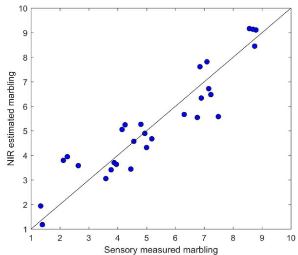
Correlation of NIR measurements with marbling as measured by the trained panel.
