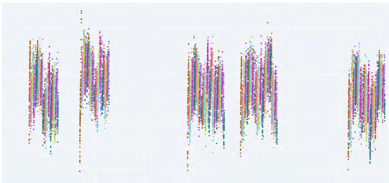
Screenshot from the Intelecy software, showing time series of dry matter in fresh cheese measured by NIR. Each dot represents a block of cheese, and colours represent different batches.
