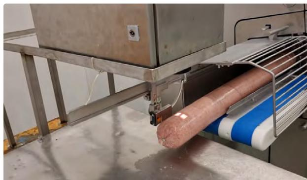
Sausage being measured with NIR spectroscopy in process line.
