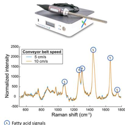
ROBOSENSE latest results in 2023: a robotic Raman scanning system for fast and effective measurements of fatty acid composition in salmon fillets.
