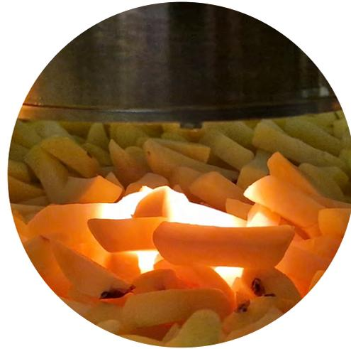
Work at Hoff during the calibration campaign in April: measuring dry matter in French fries using both interactance and reflectance NIR spectroscopy. The Perten instrument (to left in image) is currently measuring spectra continuously. The three bottom images are close-ups of measurement spots of the three instruments – Perten, Prediktor, QVision.
