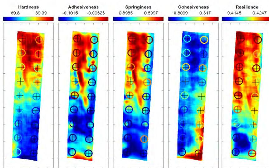
Various texture characteristics of cheese such as hardness, adhesiveness, springiness, cohesiveness, and resilience were measured using a Texture Analyzer. Afterwards, the texture parameters were estimated from the spectral data, taking the reference information into account. An example of the texture prediction maps is presented in the figure above.
